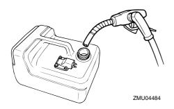
Securely close the cap after filling the tank. Wipe up any spilled fuel.
